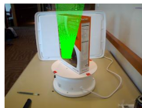
Figure 3: Planar object pose estimation using ORB.
