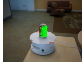
Figure 8: Non-planar object pose estimation using DARP.
