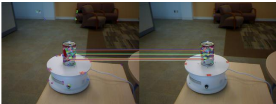
Figure 7: Non-planar object keypoint matching using DARP finds 14 matches.
