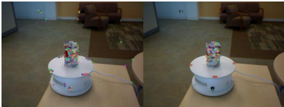
Figure 6: Non-planar object keypoint matching using ORB finds 0 matches.
